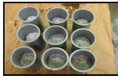
Fig. 2. Substrate concrete cylinders in the forms
