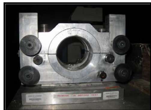
Fig. 5. Direct shear test device (LISST)
